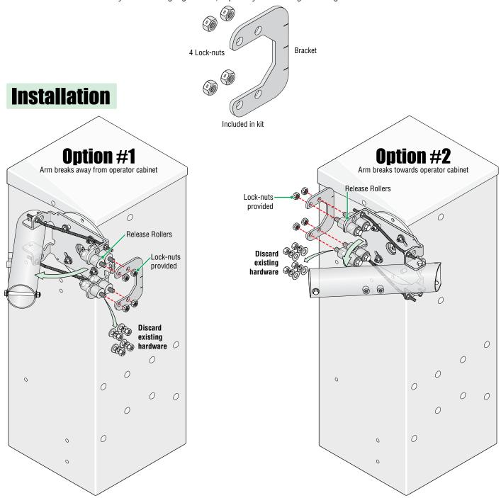
Remove the nuts, flat-washers and lock-washers from the (4) existing release roller bolts and **discard** . Mount bracket on release roller's bolts and use lock-nuts included in this kit.
