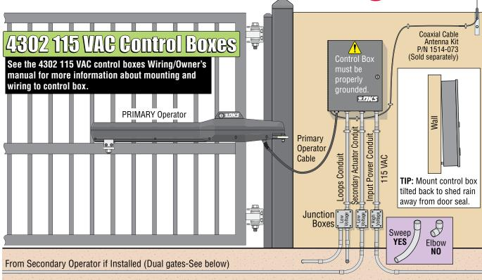
**Dual Gate Operators (115 VAC or Solar Control**
