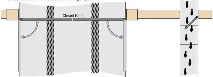
Entrapment Protection must be provided for the gate system where the risk of entrapment or obstruction exists. The operator will NOT run without one or more monitored type B1 or B2 entrapment protection devices in EACH **ENTRAPMENT AREA.**
