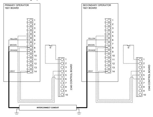
Barrier gate systems use two primary operators for bi-parting barrier gate systems. Wire barrier gate operators as shown in Figure 10. Color code shown assumes the use of DoorKing interconnection cable. Order part number 2600-755 (30 ft.), 2600-756 (40 ft.), 2600-757 (50 ft.).
